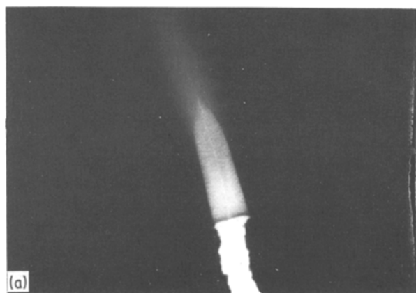
Figure 3 (a) Region of local deformation that was observed to form in response to deformation of PS that had been crosslinked to \nu_x^0 = 3.7 \times 10^{25} chains \text{m}^{-3} . (b) Region such as that shown in (a) that had been crosslinked with an additional \nu_x = 7 \times 10^{25} strands \text{m}^{-3} and then annealed above T_g .
